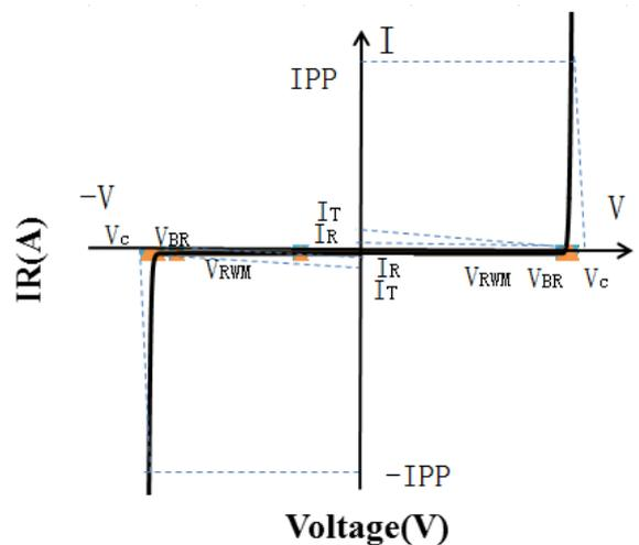
Typical Performance Characteristics ( $T_A=25^{\circ}\text{C}$  unless otherwise Specified)
